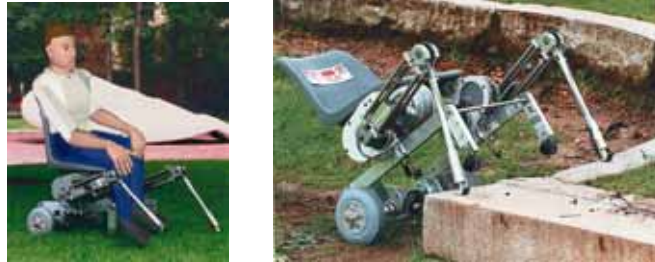
Figure 3. Prototype of chair with legs and wheels and crossing obstacles impeding the course of locomotion.
