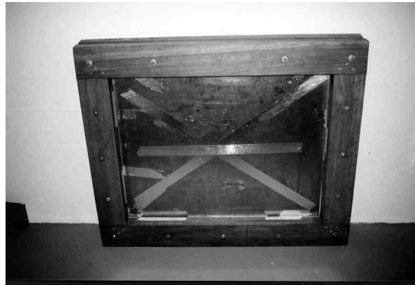
Figure 1: Wood structure built for the simply supported plate.
