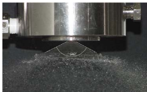
Figure 8. Fuel injector testing with water at 5 bar
