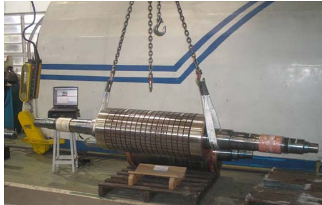
Figure 4. Rotor suspended for a free-free support condition experimental test.
