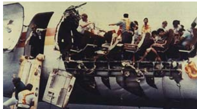
Figure 3. Fuselage separation of the Aloha Airline aircraft in 1988 (Farrar et al. , 2005).
