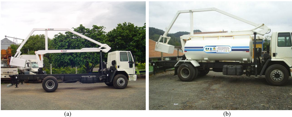
Figure 15. Robot mounted on the truck: (a) without water tank; (b) with the water tank.
