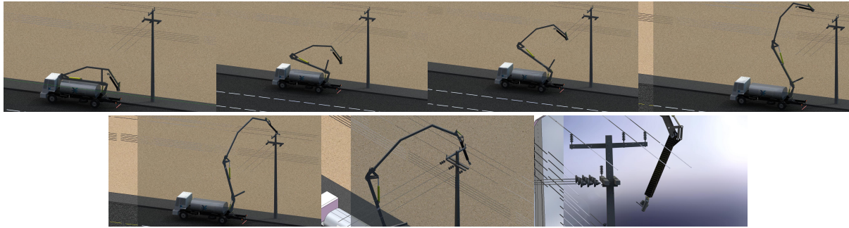
Figure 10. Sequence of the washing insulator operation.
