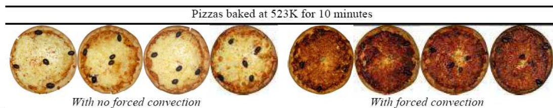
Figure 5. Pizzas obtained from step I with and without forced convection.
