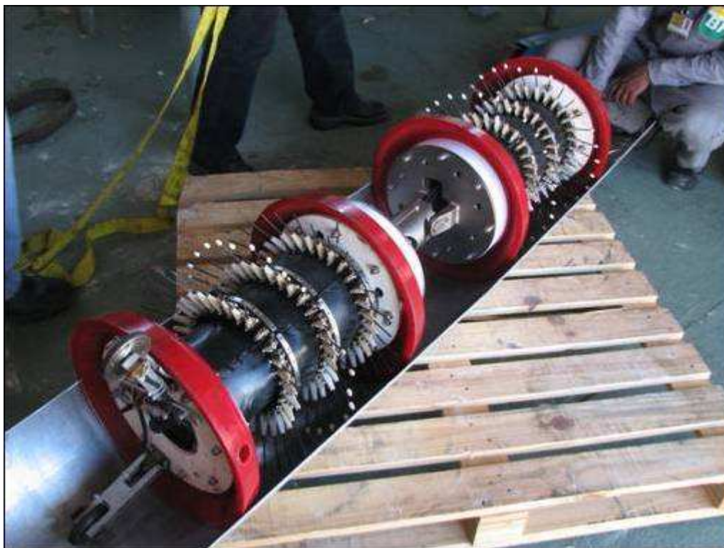
Figure 2 – The feeler pig to the pipeline by 16-diameter inches. It has 6 crowns by 30 sensors, with a total of 180 sensors. The electronics and batteries are housed within the pig.
