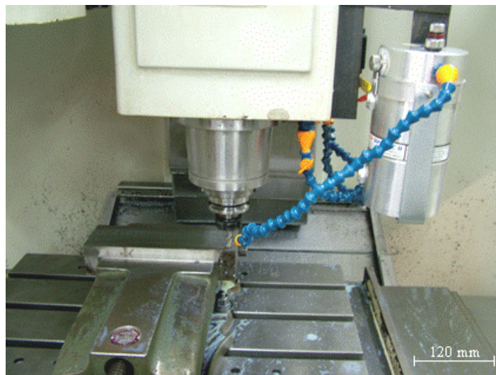
Figure 1. Picture of the milling tests with MQL application.
