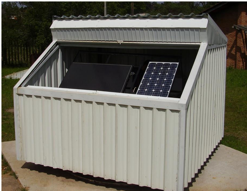
Figure 2. Climatic chamber in a PV module characterization test.
