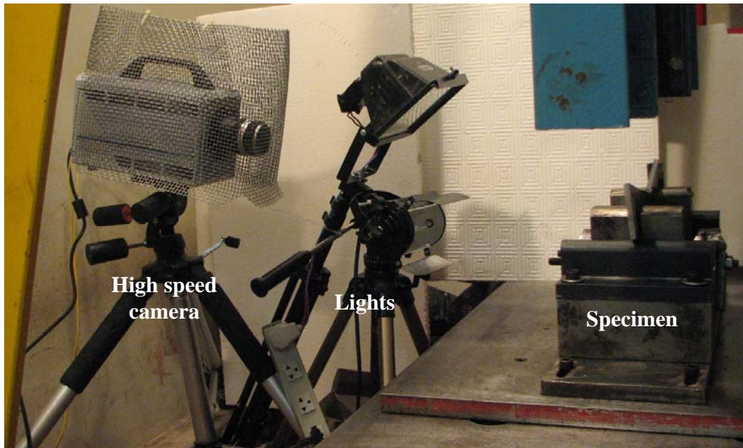
Figure 3. Recording arrangement of the DWTT test.
