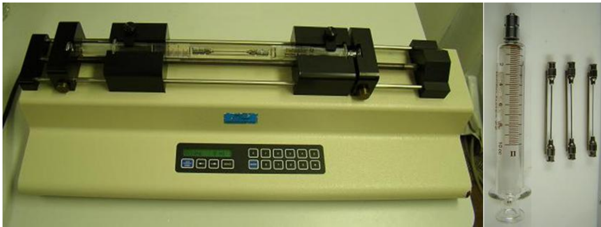
Figure 1. Experimental Setup: a) Emulsator system assembly, b) Syringe and micro-emulsifying needles.
