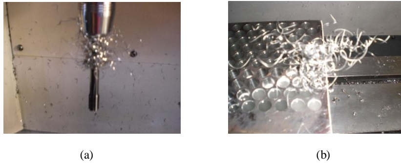
Figure 8. Curled chip on the tool shank (a) and hole obstructed (b).
