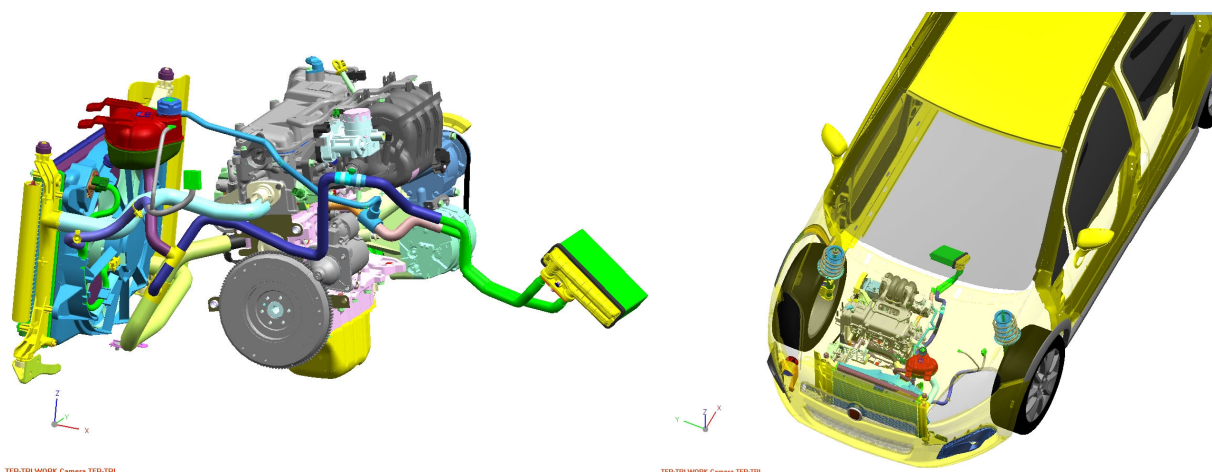
Figure 1 – Vehicle cooling system and 1.4 Fire Flex engine
