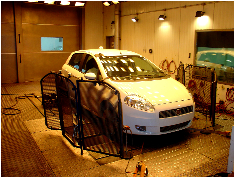
Figure 2 – Climatic chamber with roller dynamometer
