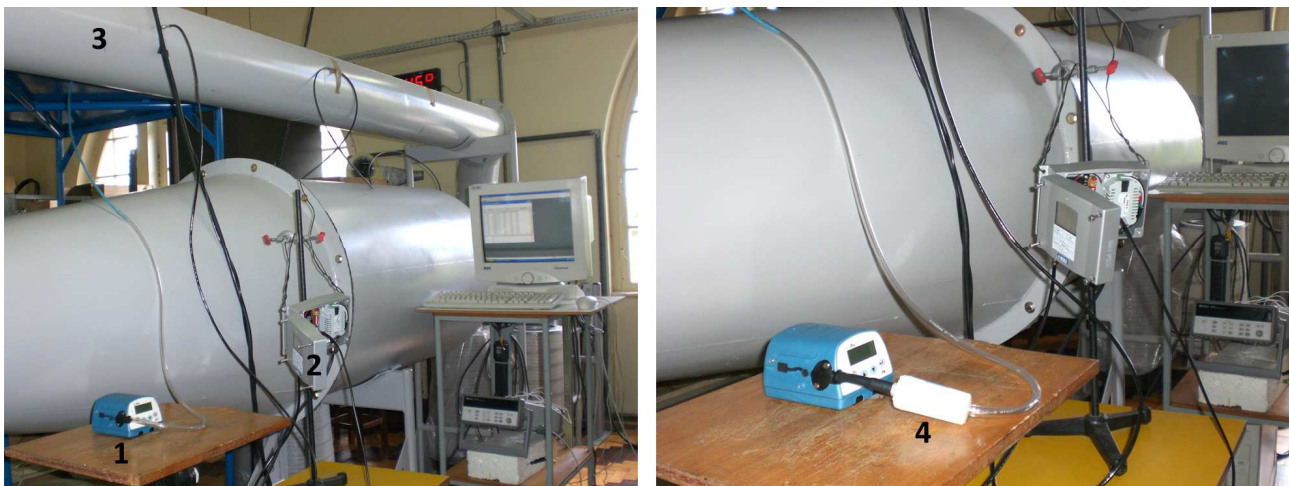
Figure 3. Filter test bench (1 aerosol monitor, 2 T and RH transmitter, 3 acquisition points, 4 monitor with built-in filter)
