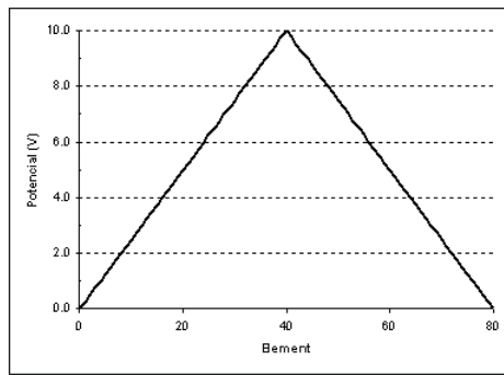
Figure 5. Triangular electric voltage excitation profile on the 80 elements of the external boundary.
