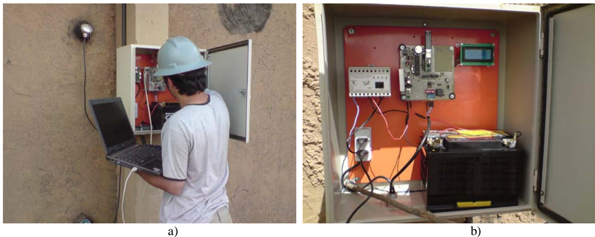
Figure 4. Acquisition system. a) Installation and configuration; b) Motherboard and components of the system
