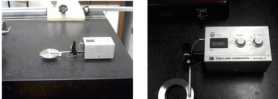
Figure 2 - Superficial roughness measurement on orifice plates
