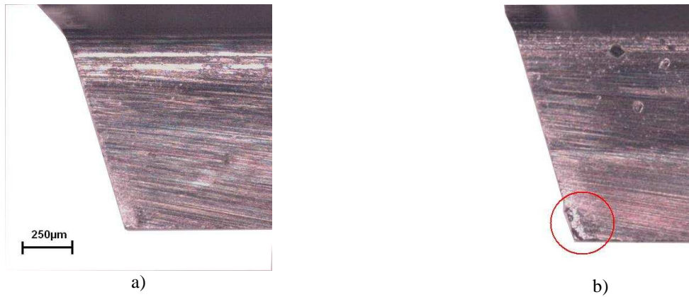
Figure 6 – Reamers; a) without adhesion; b) with adhesion
