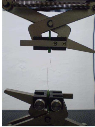
Figure 2. Tensile test for the fibre of sisal, failure.
