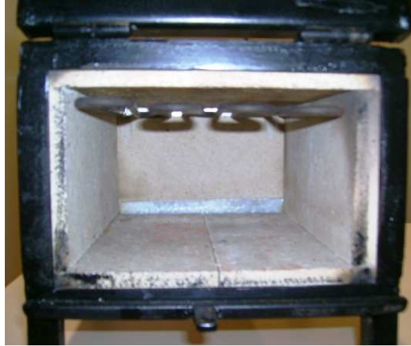
Figure 1. Detail of the resistance set at the top of the heating device
