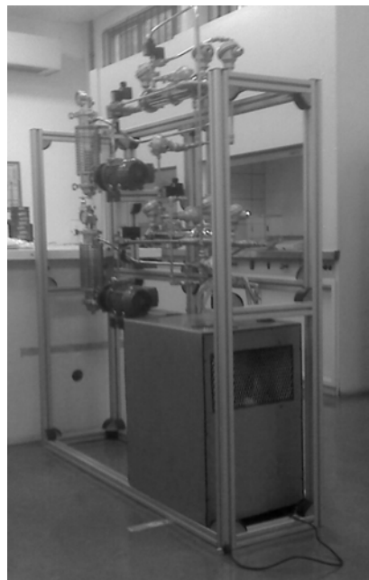
Figure 12 – Experimental apparatus: The heat exchanger network
