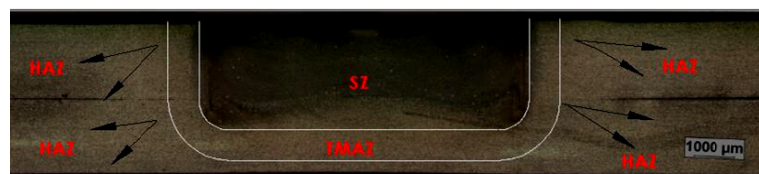
Figure 2 - Cross section of FSpW joint to Unclad AA 2024-T351, showing the limits of the weld zones.
