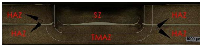
Figure 4 - Cross section of FSpW joint, to Al-clad AA 2024-T351, is showing the limits of the weld zones.
