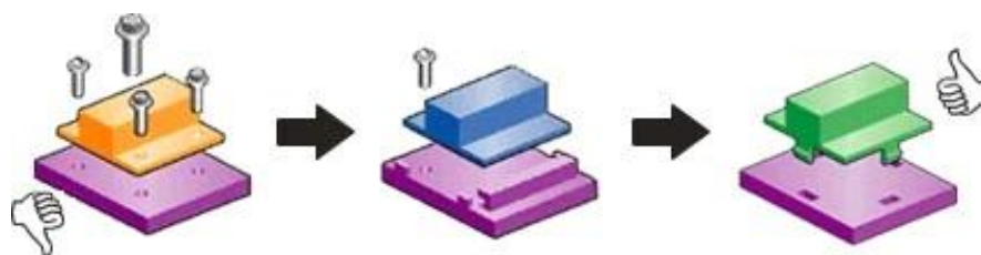
Figure 05. Comparison of the original project for the modified project of an injected plastic component, aiming at its easy assembly. (GE Plastic, 2003)
