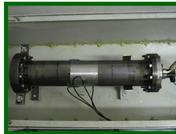
Figure 7. Specimens fixed in the test rig with supports.
