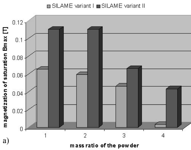
Figure 17. The influence of powder mass fraction on a) magnetization, b) coercivity H_c of composite SILAME 6:1, the powder mass fraction 1 – 6:1, 2 – 5:1, 3 – 3:1, 4 – 2:1
