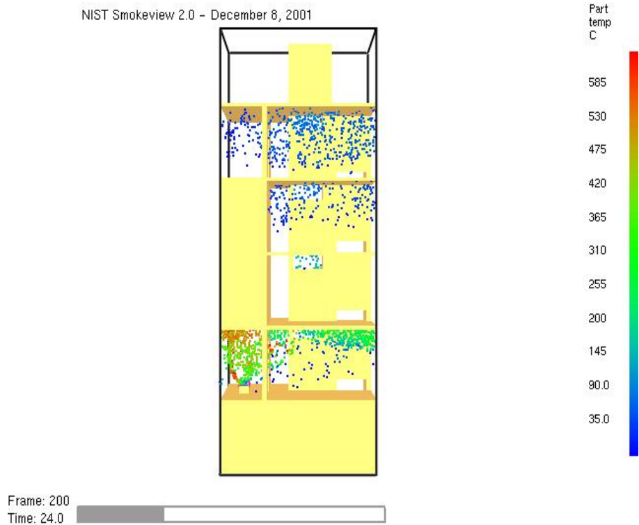
Figure 4. Case 2 - double duct: air inflow/exhaust smoke construction, particles on 24 s, 18 m building.
