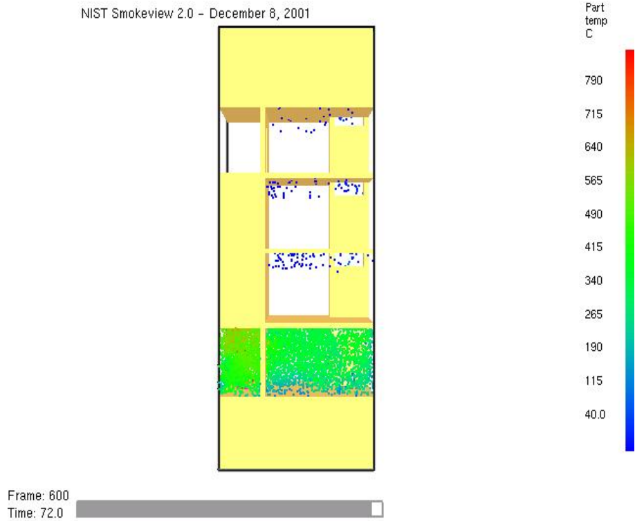
Figure 3. Case 1 - single duct: air inflow and exhaust smoke construction, particles on 72 s, 18 m building.
