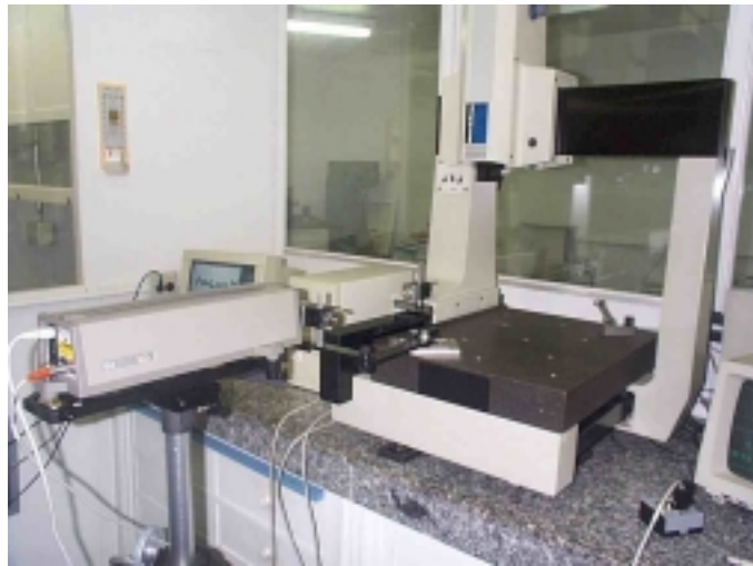
Figure 1. CMM and laser interferometer measuring system.
