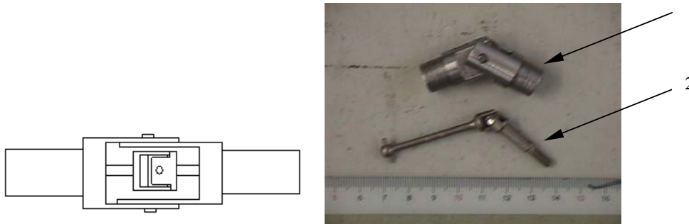
Figure14. Drawing of the wrist with universal joint and photo of the components.
