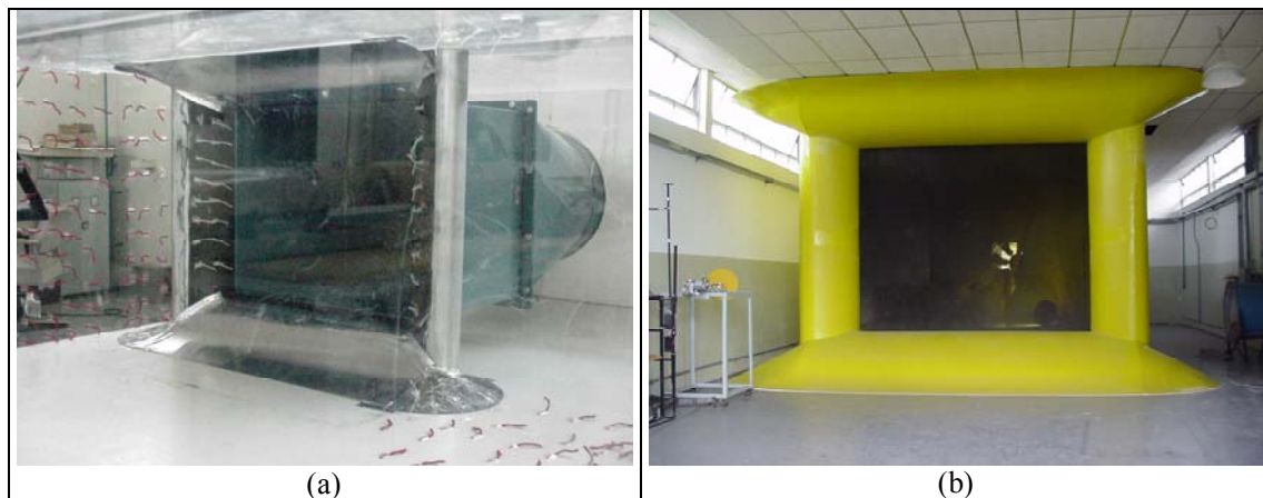
Figure 3: (a) Wind tunnel entrance and laboratory building scale model and (b) entrance nozzle of ITA's wind tunnel.
