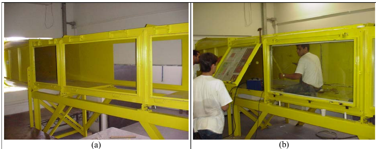
Figure 7: (a) Test section basic structure inside the sealed chamber. (b) Test section final adjustments. Assembling procedure of the transparent and opaque windows.
