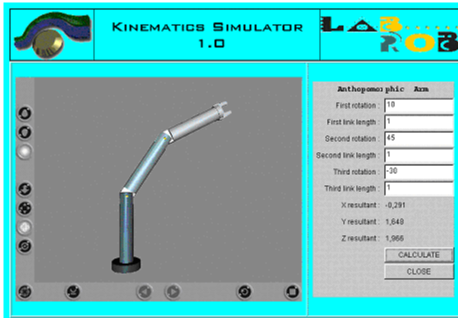
Figure 13. Anthropomorphic Manipulator shown in the VRML browser controlled by a Java applet, both incorporated in a HTML document.
