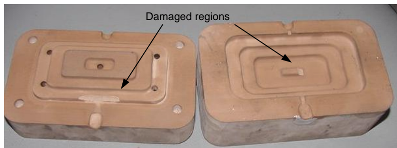
Figure 6. Damages in the inserts of the resin 460
