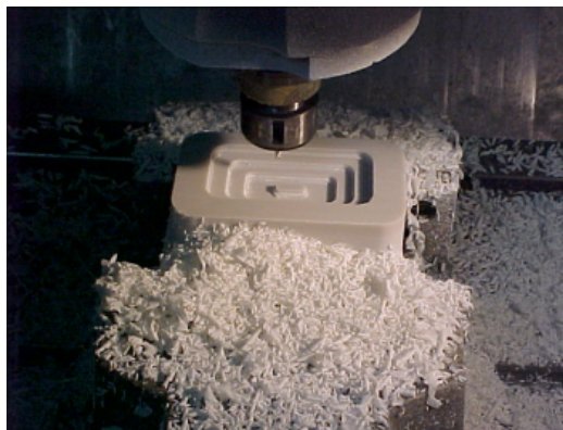
Figure 3. The CNC machining of the insert (Ren Shape 5166)
