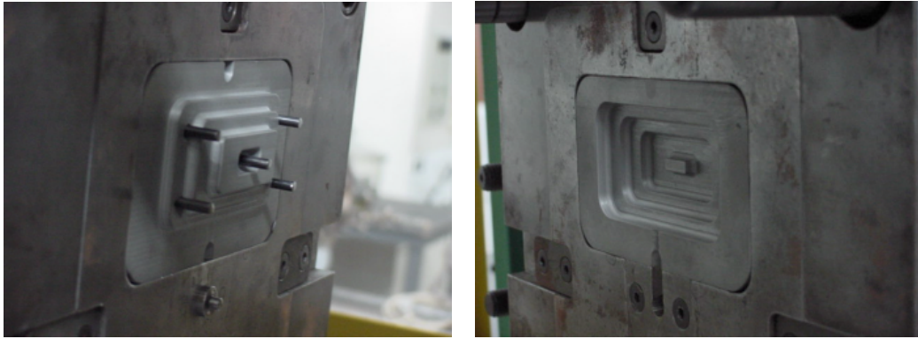
Figure 4. Core and cavity inserts assembled in the mould plates (Express 2000 inserts)
