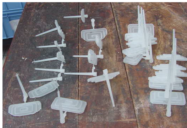
Figure 7. Some prototypes injected in the epoxy resin mould (Express 2000 inserts)
