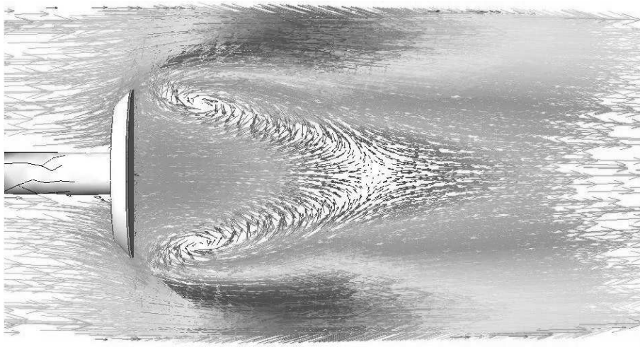
Figure 7: Confined Disc Bluff: Visualization of recirculation zone
