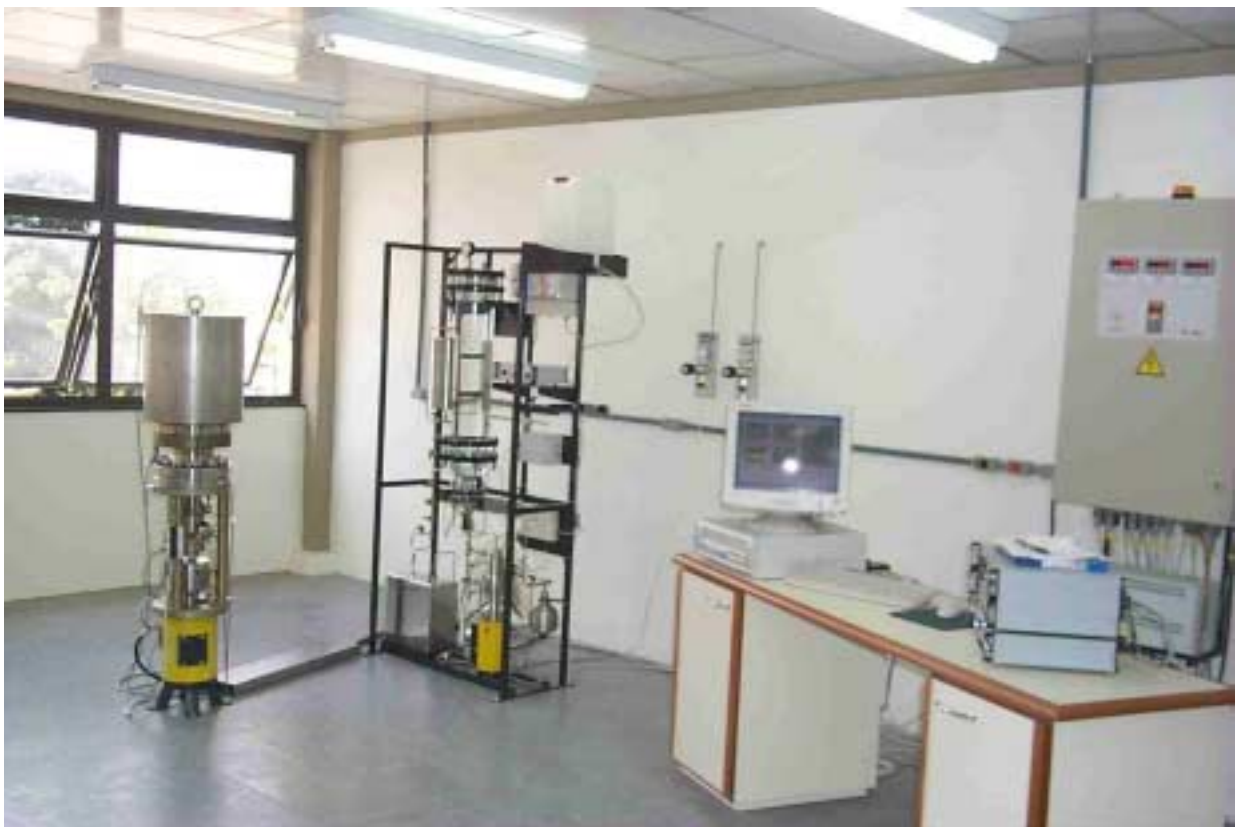
Figure 1 - Facility for stress corrosion cracking testing.
