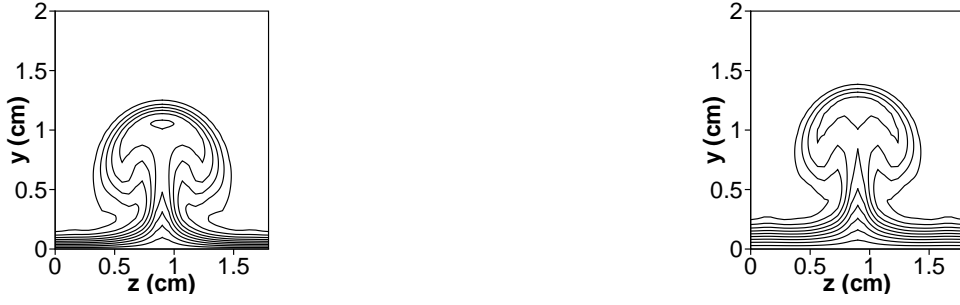
Figure 8: Contour lines of streamwise velocity u/\bar{U}_\infty from 0.1 to 0.9 in increments of 0.1. Left - type 2 buffer domain. Right - type 1 buffer domain. \Lambda_f = 450 . Streamwise position x = 110 cm.
