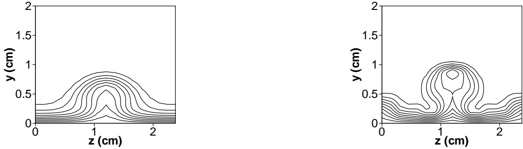
Figure 6: Contour lines of streamwise velocity u/\bar{U}_\infty from 0.1 to 0.9 in increments of 0.1. Left - type 2 buffer domain. Right - type 1 buffer domain. \Lambda_f = 692.6 . Streamwise position x = 100 cm.
