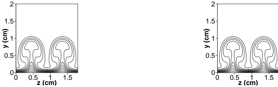
Figure 10: Contour lines of streamwise velocity u/\bar{U}_\infty from 0.1 to 0.9 in increments of 0.1. Left - type 2 buffer domain. Right - type 1 buffer domain. Streamwise position x = 100 cm.
