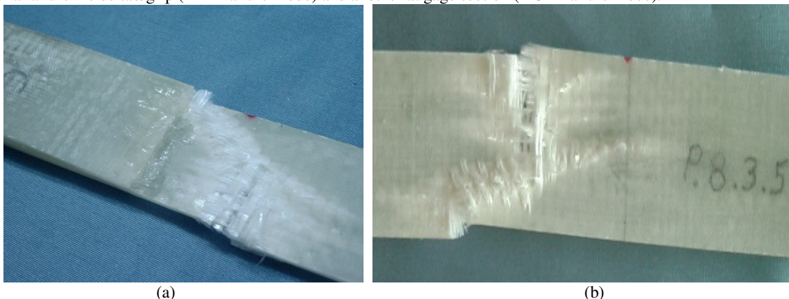
Figure 1: Failure mode on laminated composite with cure on air.
