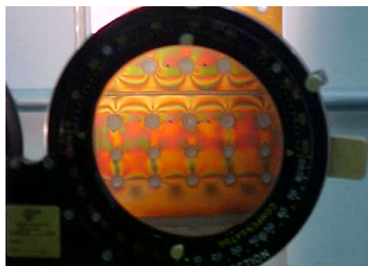
Figure 3. Isochromatic fringes for the fastened butt joint.
