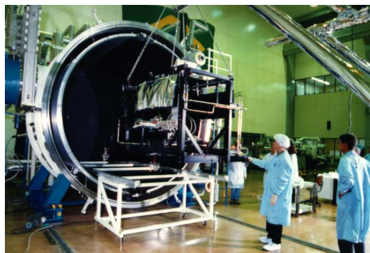
Figure 4. Adaptation of the Calibration Rig Structure in the LIT 3x3m Thermal Vacuum Chamber.
