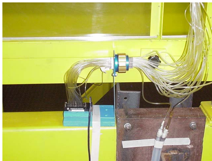
Figure 12. PSI electronic sensor mounted outside the tunnel.
