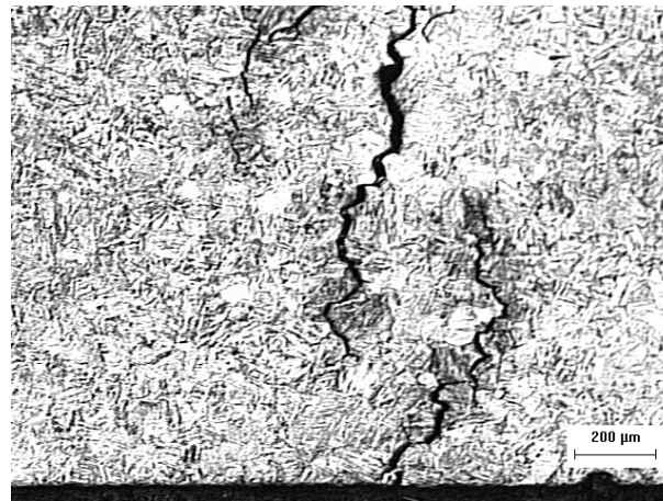
Figure 10 – Detail of internal cracks showed in Fig. (8). Etching: Vilella.
