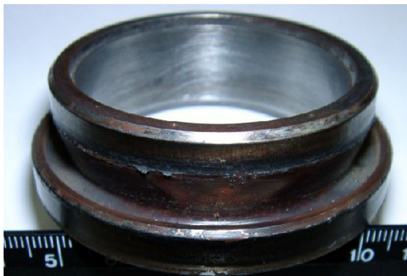
Figure 4 – Aspect in the groove region of insert 2 with corrosion product deposition.
