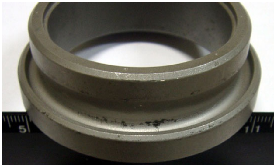
Figure 6 – Corrosion pits associated to cracks observed in insert 1.
