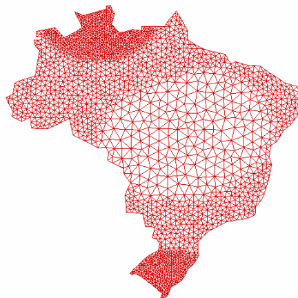
Figure 8. Top and bottom refined unstructured mesh inside the Brazil map.
