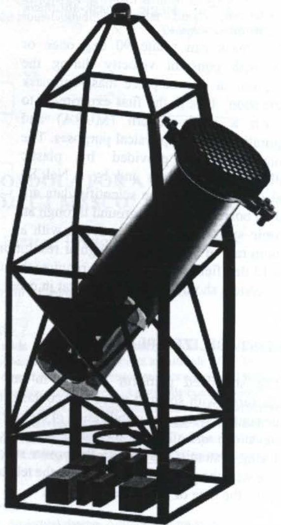
Fig. 2: The gondola of the MASCO telescope (some reinforcing beans are missing in this picture)
