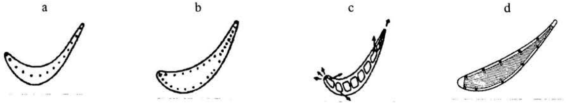
Figure 1. Cooling systems for gas turbine blades
