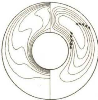
Fig. 2: Isotherms and streamlines for A = 2.2 \times 10^9 , B = 0.8 , T_i = 0^\circ\text{C} and T_o = 4^\circ\text{C} .
