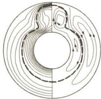
Fig. 3: Isotherms and streamlines for A = 2.2 \times 10^9 , B = 0.8 , T_i = 0^\circ\text{C} and T_o = 6.5^\circ\text{C} .
