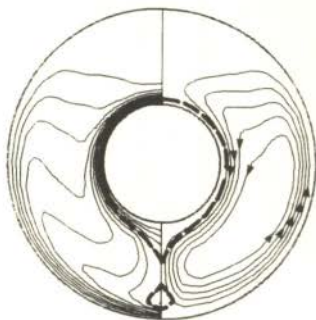
Fig. 5: Isotherms and streamlines for A = 2.2 \times 10^9 , B = 0.8 , T_i = 0^\circ\text{C} and T_o = 12^\circ\text{C} .
