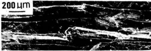
Fig.1: Slip markings in Mg matrix of Mg/B. 2000 cycles, 280 to 40°C.
