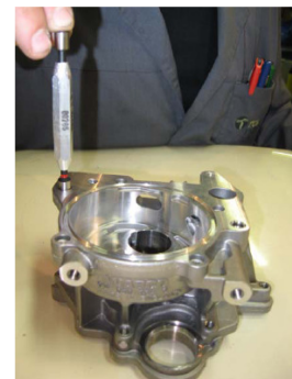
Fig. 5: Pin bore inspection
