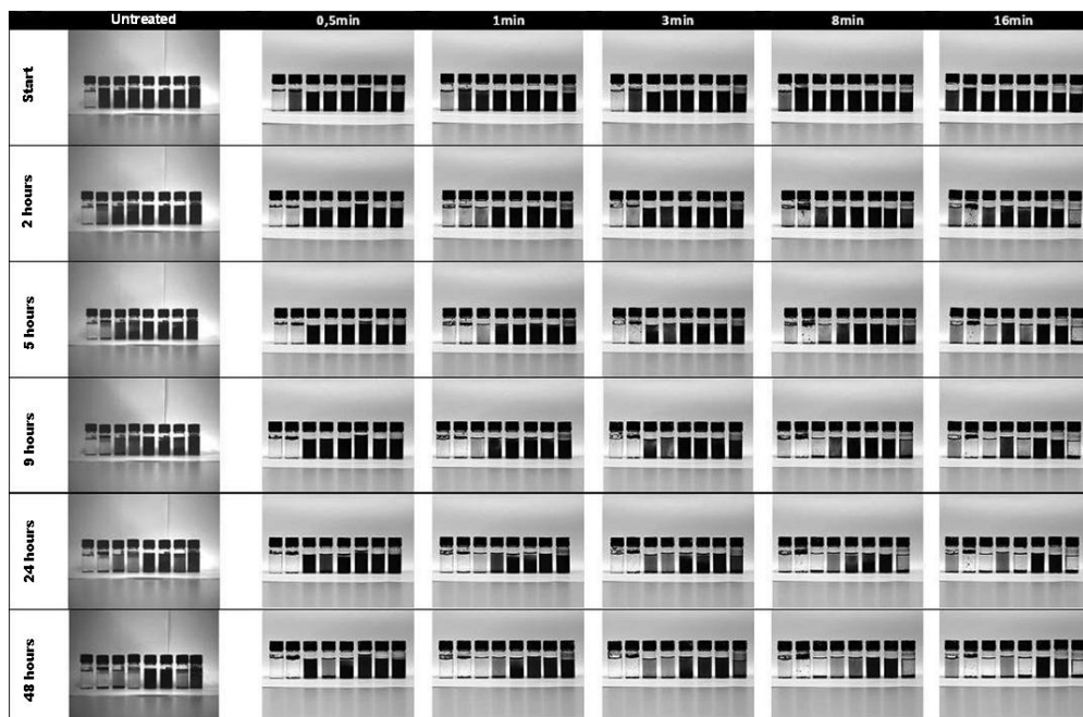
Figure 5. Images of sedimentation behavior tests to MWCNTs in solvents as function of time treatment under oxygen plasma. The solvent order from left to right is: water, hydrogen peroxide, isopropyl alcohol, acetone, DMSO, DMF, THF and chloroform.
